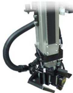
Example of a servo-driven rotational B/C axis
